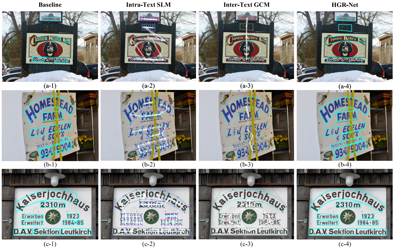
Fig. 7. Qualitative detection results of baseline, Intra-Text SLM, Inter-Text GCM, and HGR-Net. The centroids of detected text instances and components are connected by learned graph edges. Edge thickness corresponds to scaled edge weights.
